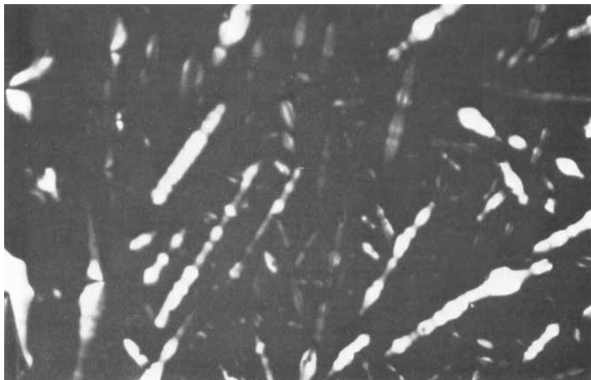
FIGURE 2 : Formation of bâtonnets occurring in the system a prior to phase separation ; crossed polarizers (Gx280)
