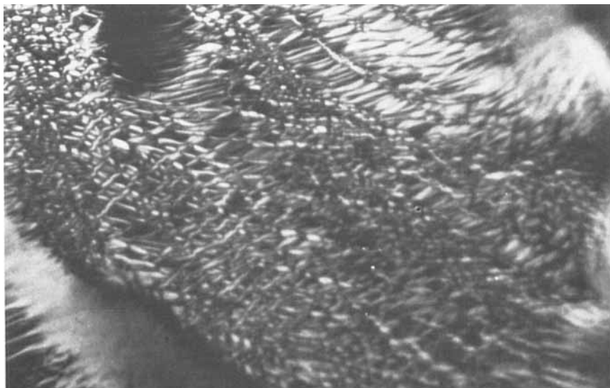
FIGURE 4 : Mosaic texture in a lamellar phase (system b) ; crossed polarizers (Gx580)
